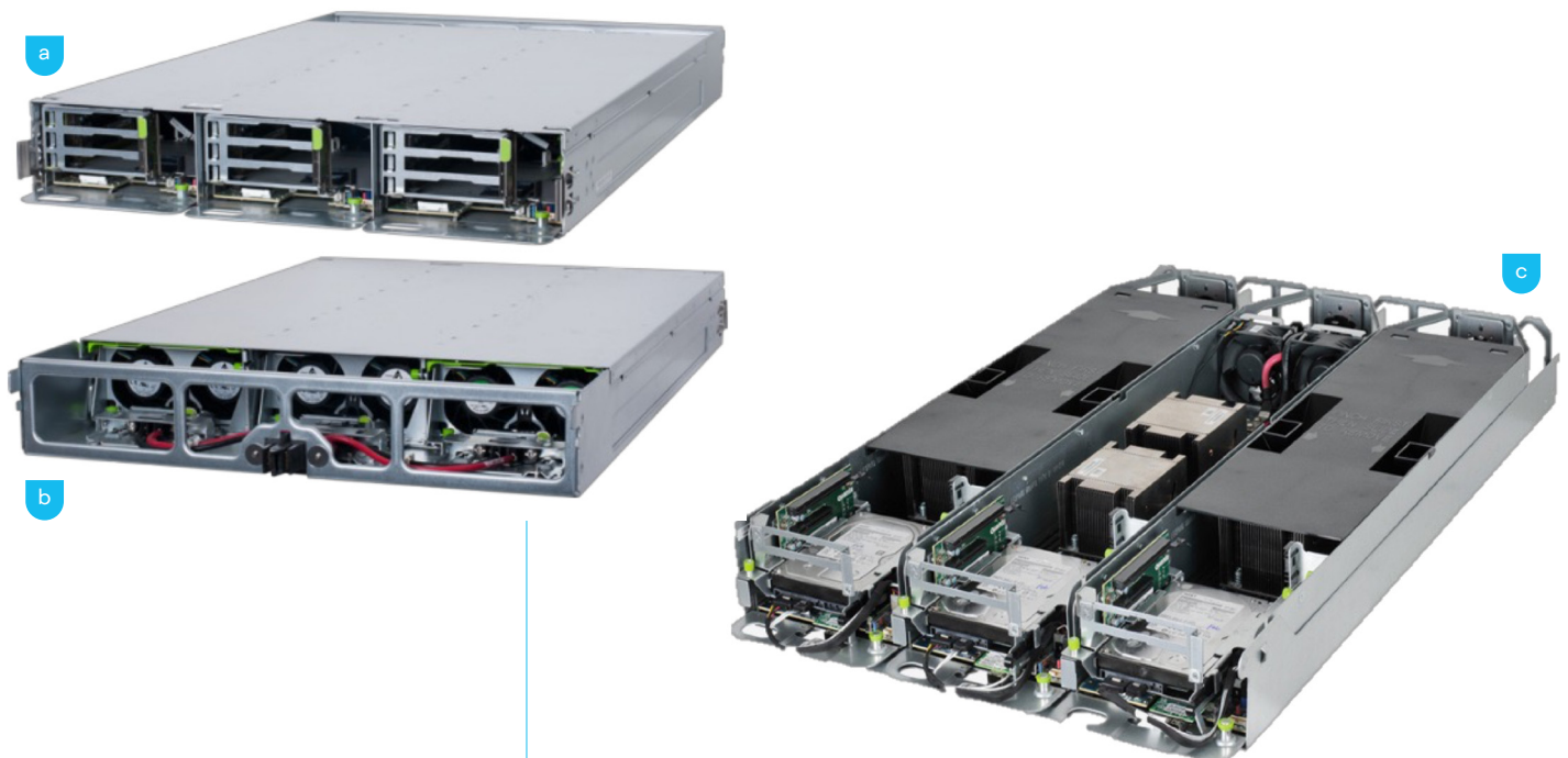
Figure 1. As-delivered stock OCP Leopard Servers in Open Rack V2 Cubby (a) front view, (b) back view, and (c) Internals of stock OCP Leopard Servers.
